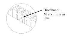
We advise to all users to fill the burner only to the bars mark ( like you can see in the picture) Its capacity is define to support 2 litres.
