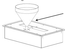
To filling the burner you have to push down the fuel cover.
